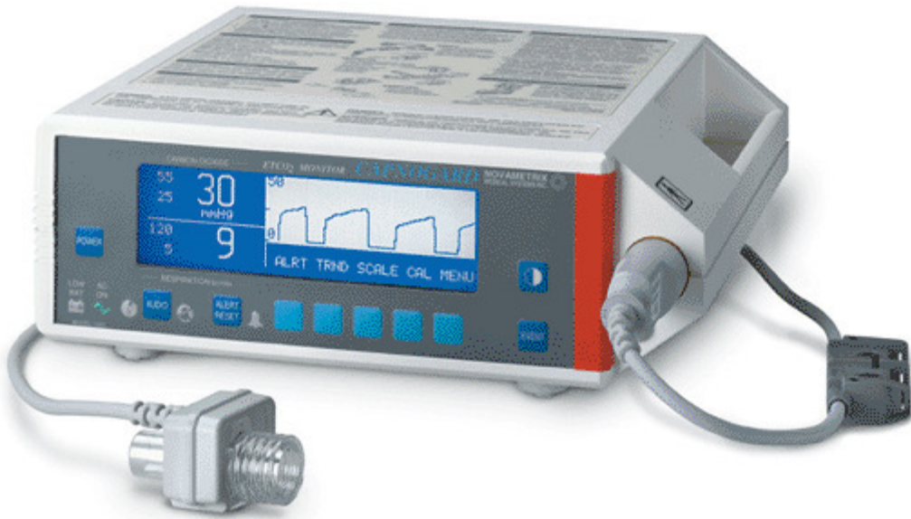
FIG. 10.1. Mainstream capnographic monitor unit and clip-on sensor assembly. (Courtesy of Respironics, Inc., Murrysville, PA, USA.)
