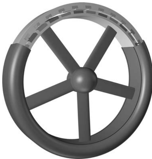
Figure 2.12 Integration of a rim-generator in a TEC
