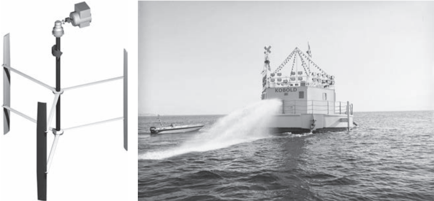
Figure 2.11 Kobold turbine: (left) scheme of turbine rotor and electrical generator; (right) prototype device, driving a pump to dissipate the generated power (reproduced by permission of Ponte di Archimede International Spa)
