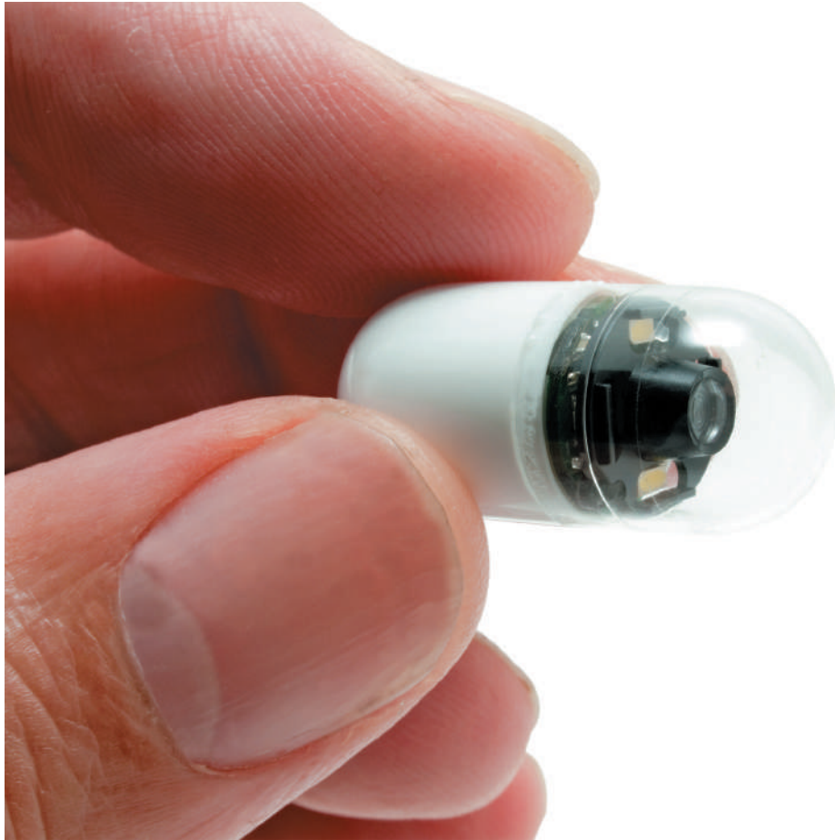
FIGURE 8.17 The capsule endoscopy camera is swallowed by the patient so that it can transmit images from the small intestine to a sensor device.
