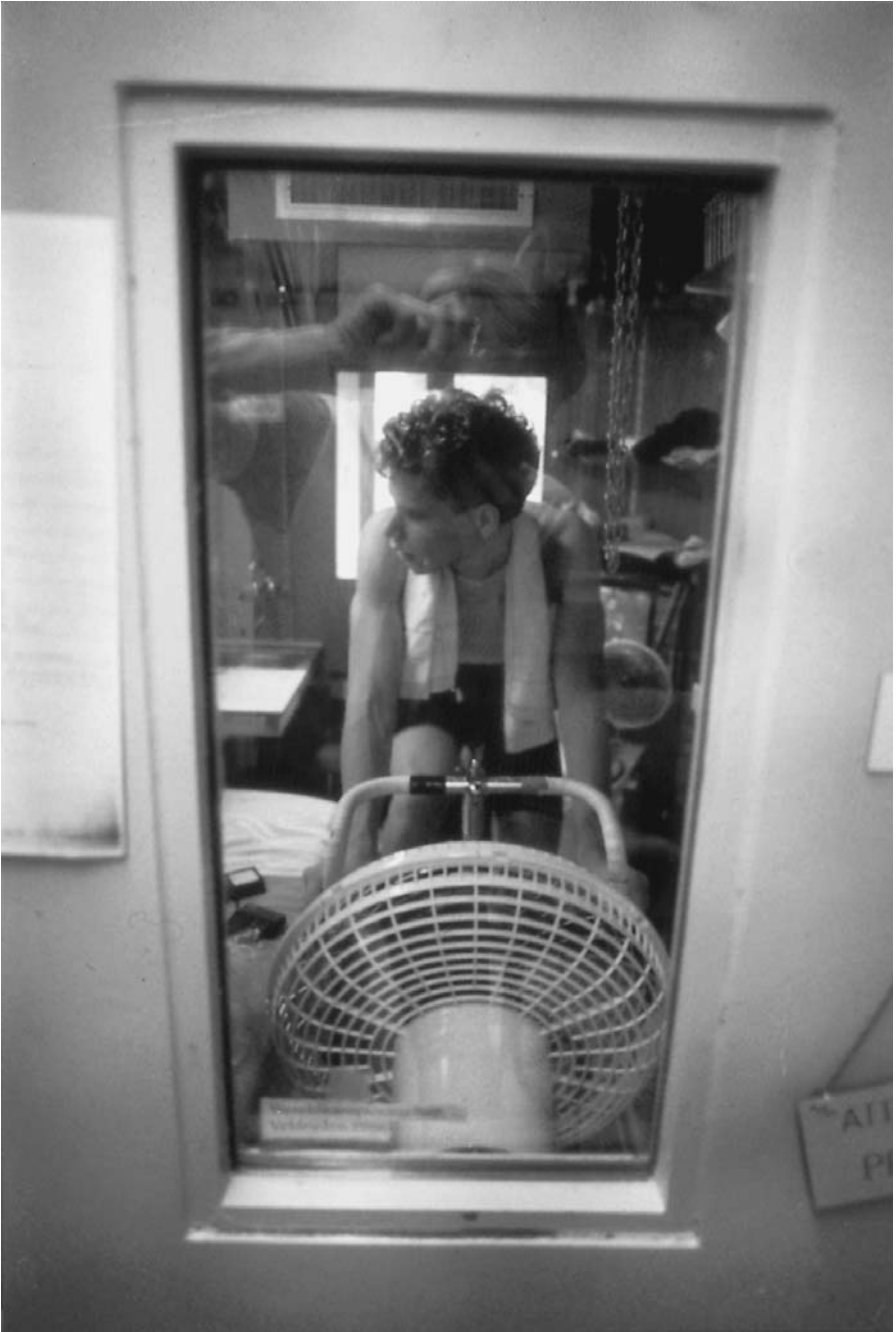
Figure 14 A six day Tour de France simulation experiment in a respiration chamber at the Maastricht University, Maastricht, The Netherlands. Indirect calorimetry allows continuous measurement of energy expenditure
