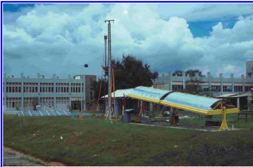
Figure 8. Wrede solar-thermodynamic pump and PV pump on test at INDOTEC, Santo Domingo, Dominican Republic, 1984.
