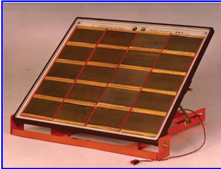
Figure 3. A French PV generator of CdS from 1973.
