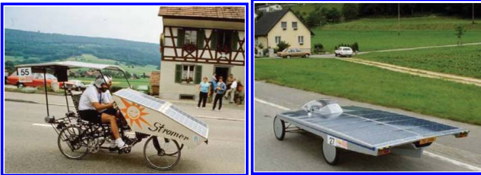
Figure 2. The solar bicycles and solar cars of the world first Tour de Sol 1985. Left: Supplementary to PV solar energy, some of the solar cars were powered by pedals. Right: The winning solar car of Mercedes/Alpha Real won the first Tour de Sol from the lake of Constance to the lake of Geneva in 1985 with a velocity of 70 km/h.
