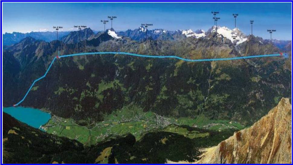
Figure 47. Proposal of the Swiss Greina Foundation of 2007. The figure shows the planned 1000 MW water power plant (actually 43 MW) in Poschiavo, Grisons, with a new power line of 17 km length between Lake Poschiavo (left/950 m) and Lake Bianco (right/2250 m). With this project, hydro-peaking (S-SV) is decreased from 1:24 (respectively 1:40 as planned in 1995) to 1:2. The concrete dam at the Bernina is only augmented by 4.3 m instead of 17 m, and conforming residual water quantities are guaranteed. The production of regulating energy increases from 120 GWh/a to 2500 GWh/a. Thanks to 20 times higher regulating energy reserves, a 100% security of supply for PEB can be guaranteed.
