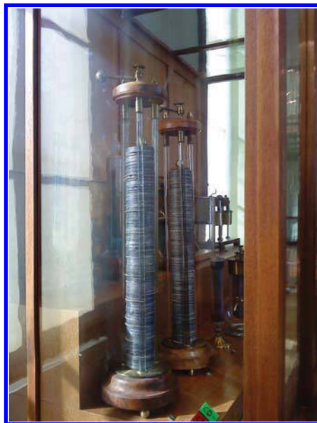
Figure 1. The beginning of electricity in the service of mankind: Volta’s electrochemical pile of zinc and silver pallets as shown in 1800 to Napoleon, a big event in those days. The picture illustrates why it is called a “pile”. Accordingly, some French people still refer to a solar cell as a “photopile”.
