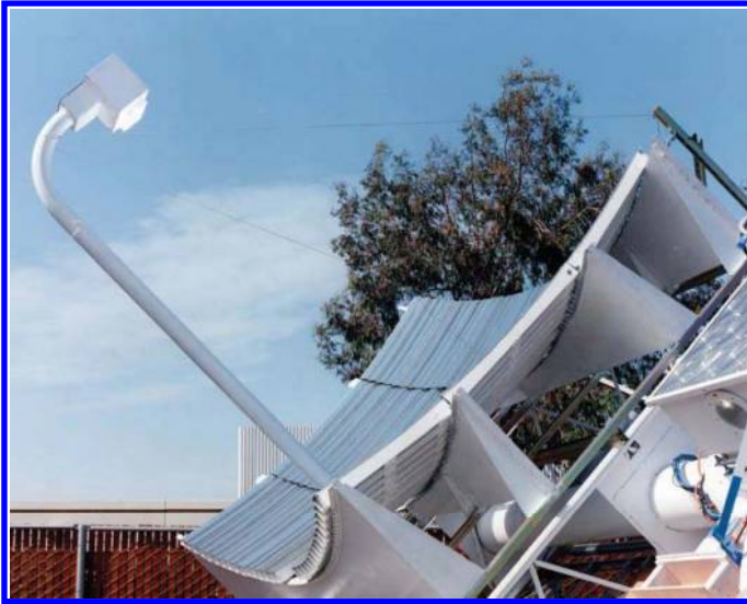
Figure 2. SunPower's dish concentrator test in 1992. Glass mirrors focus light on the cells, which are located in the receiver at the end of the boom.
