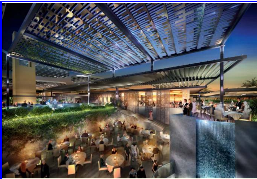
Figure 13. The roof of each building in Masdar will incorporate photovoltaic cells, supplying power directly to the city's grid. The use of shading and colonnades helps give respite from the sun and was influenced by traditional Arab settlement. Narrow streets with angled facades together with planting and water also help mitigate the fierce desert sun.
