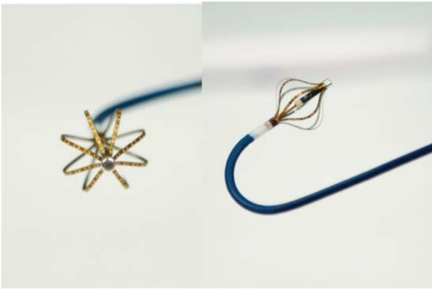
FIGURE 1-10 New micro basket catheter from Rhythmia (Boston Scientific). This catheter has a small, flexible basket with 64 poles on 8 splines using small (0.4 mm) low impedance electrodes. It also has bidirectional steering.
