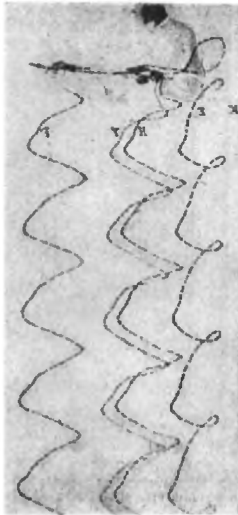
Fig. 9. A kymocyclogram of filing. The figure of the subject is visible at the top of the illustration, with a standard cyclogram of a single cycle of the movement of filing. This can be seen to be quite unanalysable. Below is a series of curves of the same movement, separated by being photographed on a moving film. K , a control bulb; E , the elbow joint; H , the radial side of the wrist joint; F , the fingers of the right hand; F' , the fingers of the left hand. Frequency - 73 frames per sec (1923).
