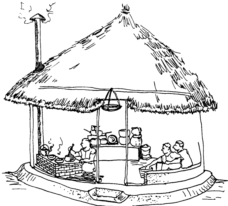
Diagram of cooking hut with chimney stove.
