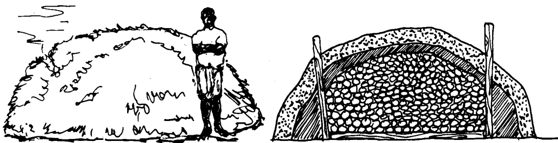
Simple earthen kilns dominate charcoal making in developing countries.
