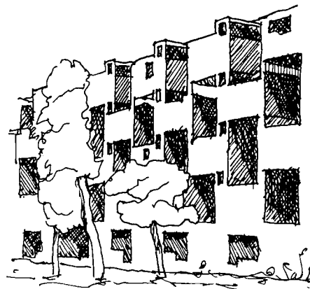
Balconies for shadowing.
