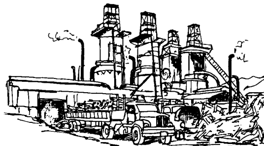
Lime boiler in Brazil, fuelled by direct heat gasifier.
