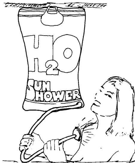
Plastic bag solar water heater used for shower.
