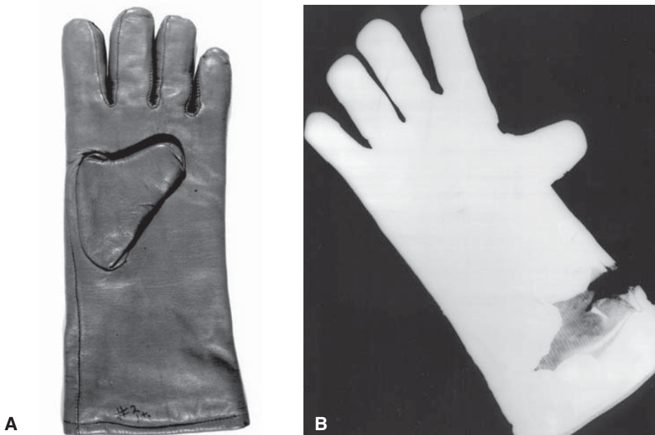
Figure 15.12. (A) Shows a photograph of a normal-appearing lead glove. (B) Shows a radiograph of the same glove that shows a gap in the protection because the internal lead shielding is torn and shifted.
