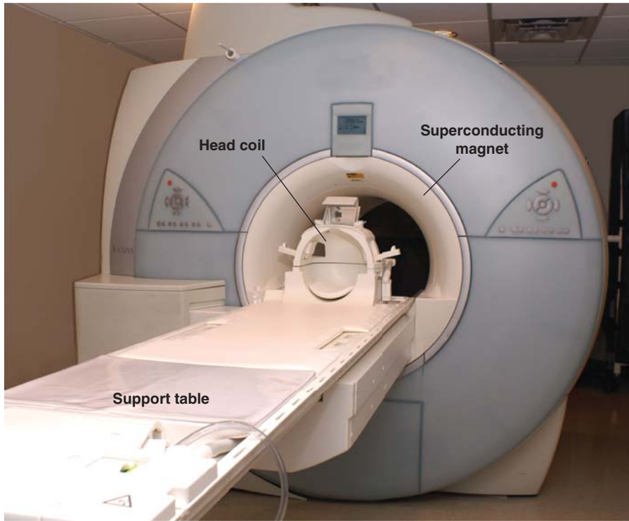
Figure 18.9. A superconducting MRI unit with a surface coil designed for MR scans of the head on the support table. The superconducting coils, which have zero electrical resistance, are surrounded by liquid helium in a dewar to maintain them at a temperature below 9.5 K.
