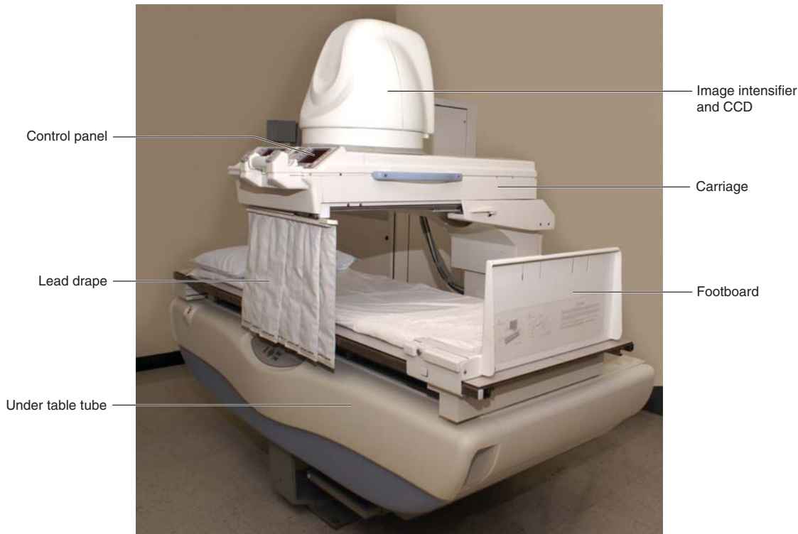
Figure 13.2. Shows a modern “R and F” room.
