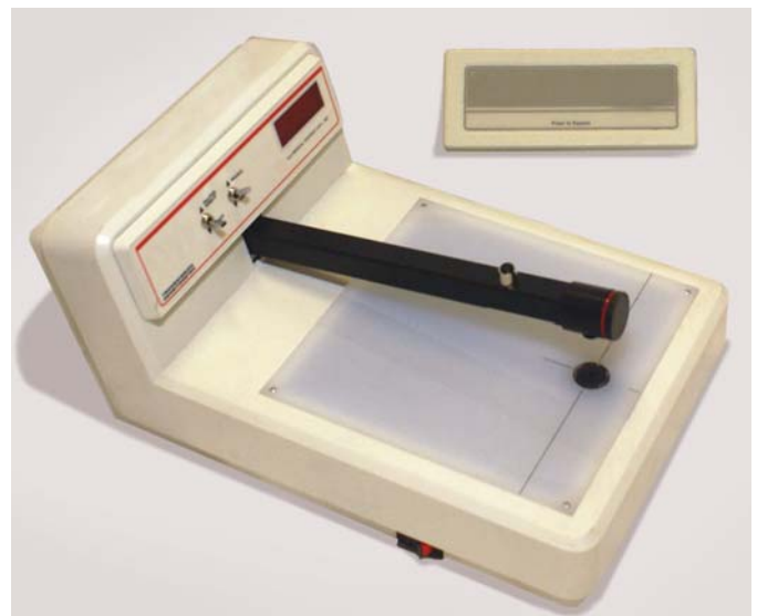
Figure 10.2. Optical densitometer used to measure density on a film.
