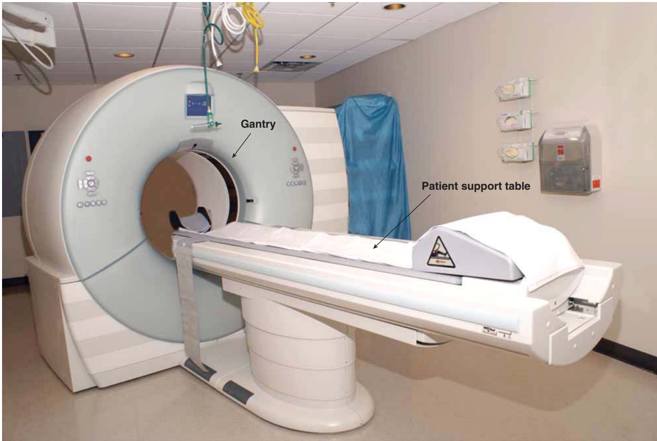
Figure 17.9. Shows the gantry and patient support table of a modern CT scanner.
