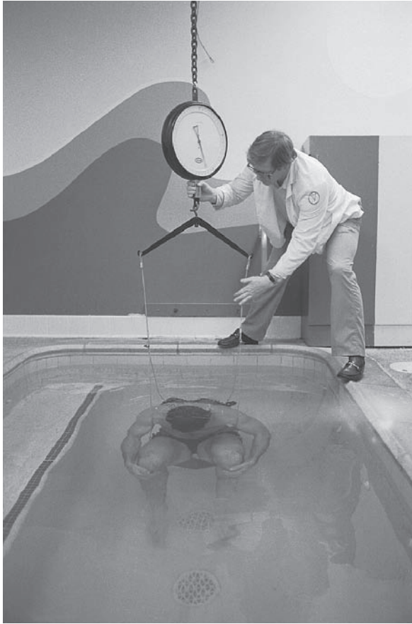
Figure 8-17 Hydrostatic weighting is the preferred method for determining percentage of body fat, but this technique is not practical as a field-test measure.
