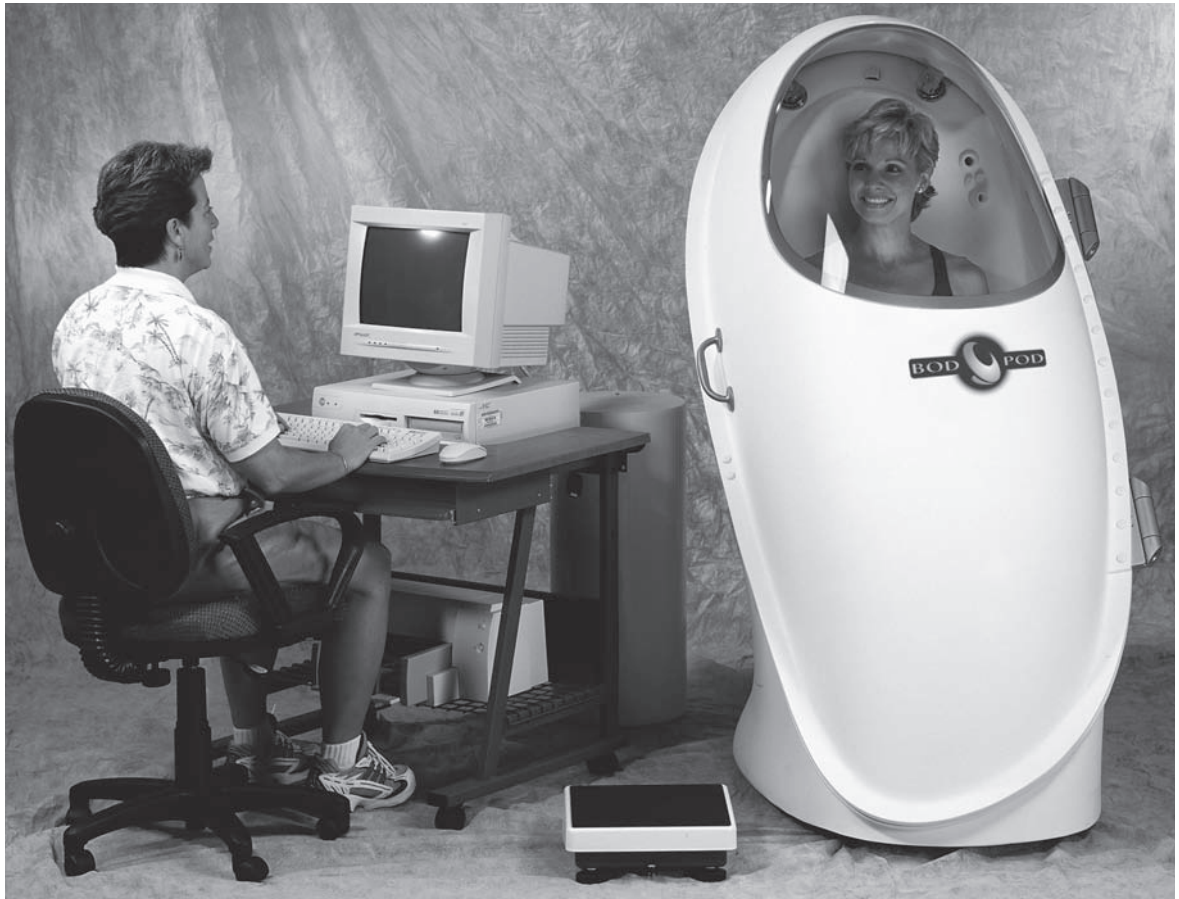
Figure 8-18 The Bod Pod uses air displacement technology to measure body composition. Image courtesy of Life Measurement.
