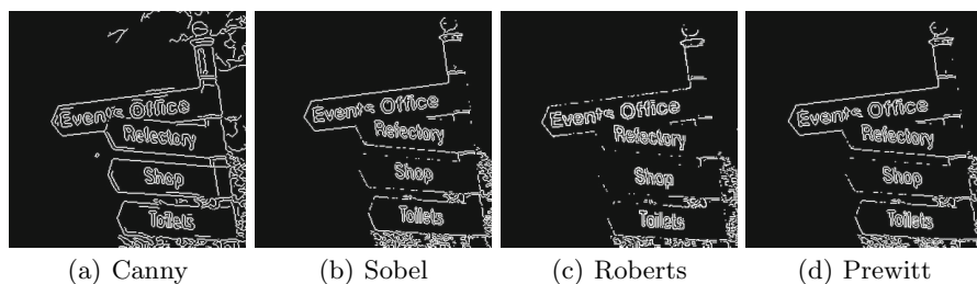
Fig. 6. Edge detection using different operators, each with perceptually optimum threshold values
