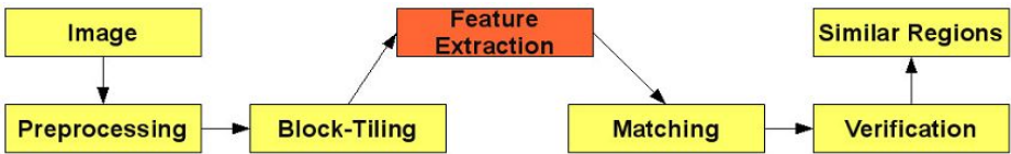
Fig. 4. The copy-move forgery detection algorithm pipeline
