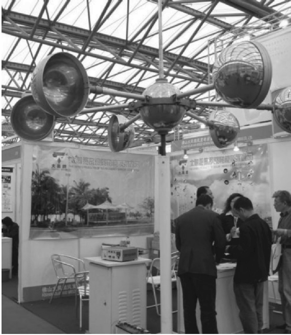
FIGURE 9.6 Drag device with cup blades, similar to anemometer. (Photo by Charlie Dou.)
