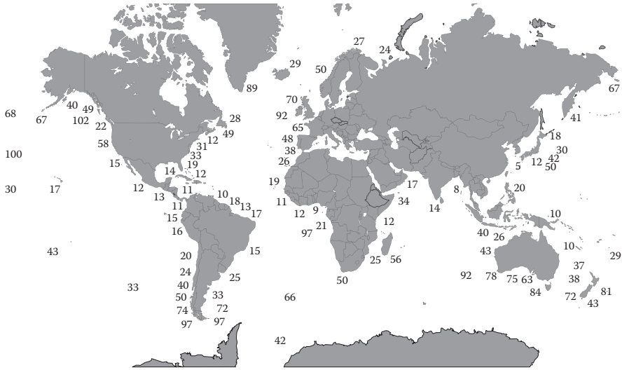
FIGURE 12.18 Average wave energy (kW/m) for coastlines around the world; values are for deep-water sites. (Courtesy of Pelamis Wave Energy.)
