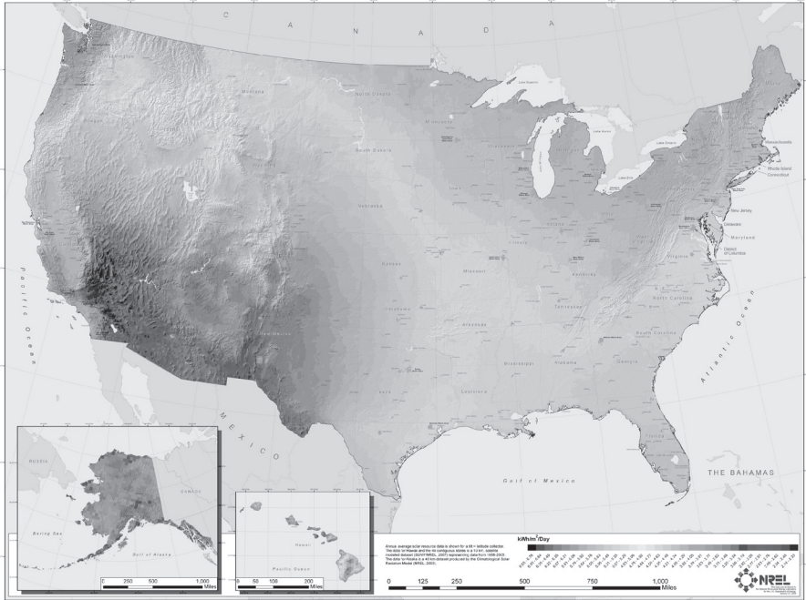
FIGURE 3.16 Solar map for the United States, flat plate tilted at latitude. (From National Renewable Energy Laboratory (NREL), Dynamic Maps, GIS Data and Analysis Tools, Solar Maps, http://www.nrel.gov/gis/solar.html .)
