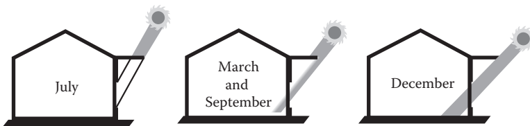
FIGURE 5.4 Overhang gives shade in summer and permits direct solar radiation into the structure in winter.
