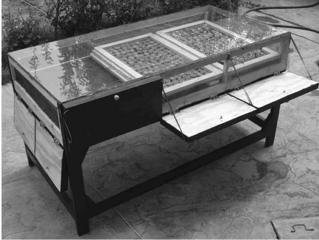
FIGURE 5.21 Direct solar dryer for fruit and vegetables, Kabul, Afghanistan. Solar dryer designed by Robert Foster. (Courtesy of Robert Foster.)
