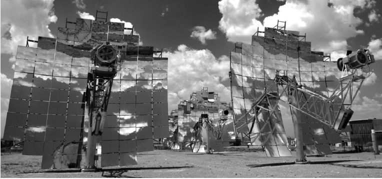
FIGURE 7.13 Test field for dish/engine at Sandia National Laboratories. (Courtesy of Sandia Labs.)
