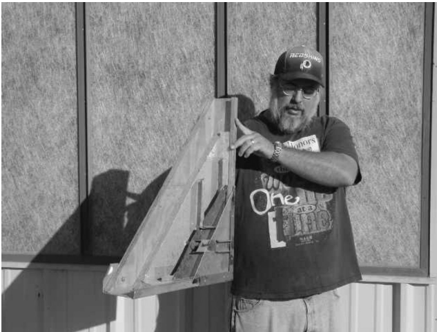
FIGURE 5.17 Cross section of vertical hot air collector. Actual collector is in the background. From outside, fiberglass glazing, dead air space, absorber plate (selective coating), air channel, insulation with aluminum foil, plywood, and metal frame. Notice that glazing on the actual collector has become more translucent with UV aging. Light transmission is still about the same.
