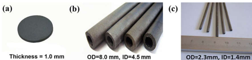
Fig. 1.4 Typical images of the plate, tubular, and hollow fiber MIEC membranes
