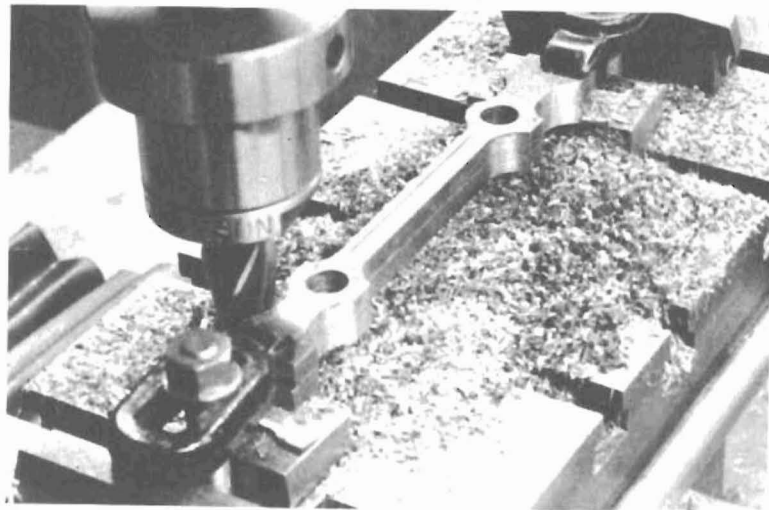
Fig. 33 Profiling coupling rods
