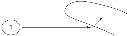
Figure 13.3 Simulating the effects of wind on airplane wing. If air molecule 1 struck the wing, the computer would calculate the precise force it would exert, and the computer would perform similar calculations for all the other air molecules striking the wing at that moment. By summing the effects of all these molecules, the computer could calculate the overall effect of the wind moment by moment, and how it would change the position of the wing.
