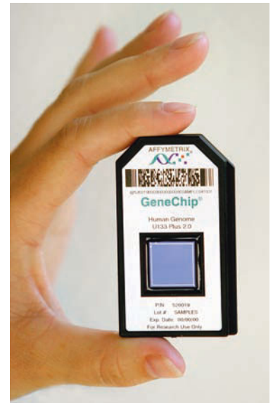
▲ FIGURE 14.12 A commercial DNA array known as a DNA chip. Each chip has between 50,000 and 500,000 fields.
