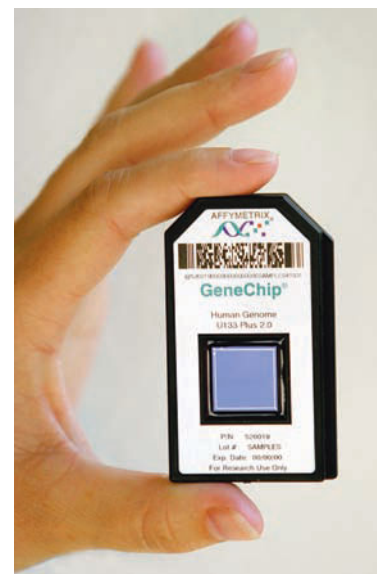
▲ FIGURE 1.11 A gene chip carrying the human gene set. This chip can be used to diagnose genetic disorders.
