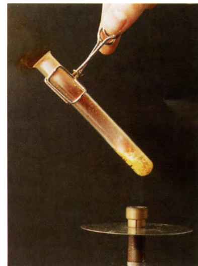
Figure 11.13 The evolution of \text{NO}_2 on heating lead nitrate.
