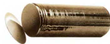
Figure 3.2 Ultra-pure silicon used for making computer chips.
