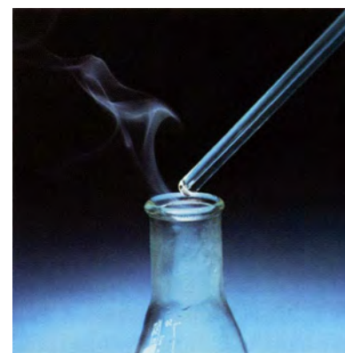
Figure 11.10 A white ‘smoke’ of ammonium chloride produced by the reaction of ammonia, in the flask, with hydrochloric acid on the rod.
