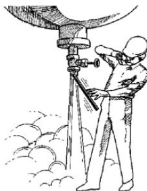
A wire or rod should never be used to unplug a drain under pressure
