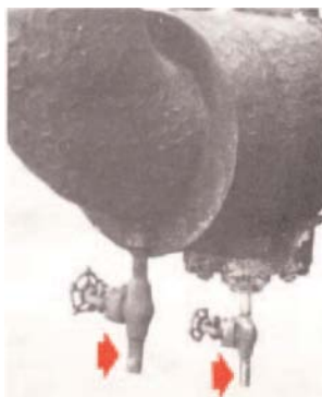
Figure 26 When drainage is complete on vacuum units, drains should be plugged or blinded to prevent entrance of air.
