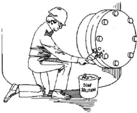
Figure 25 All leaks must be stopped before the unit is started.
