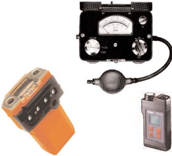
Figure 5 Combustible gas indicators operate on either the combustion principle, the thermal conductivity principle, or on infrared principle. To read percent hydrocarbon directly, they must be calibrated for the gases involved, and the proper scale must be used.
