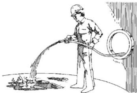
Figure 12 Pyrophoric iron sulphide must be kept wet.
