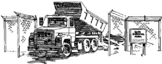
Figure 15 Burn pyrophoric iron sulphide at a safe distance from units.
