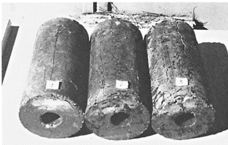
Fig. 3. Specimens held in the aggressive solution partially submerged: 1. without fibres; 2. SFRC; 3. SRFC with calcium nitrite.
