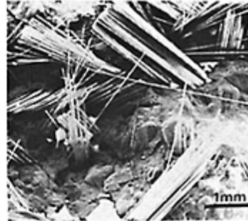
H Fracture surface of Cem-FIL 2/ grc naturally weathered for 9 years
