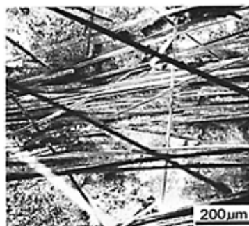
B Fracture surface of grc kept for 20 years in dry air (40% rh) at 20°C
