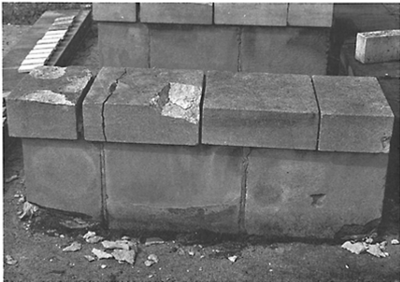
Plate 2. Frost damage attributed to the entrainment mechanism.
