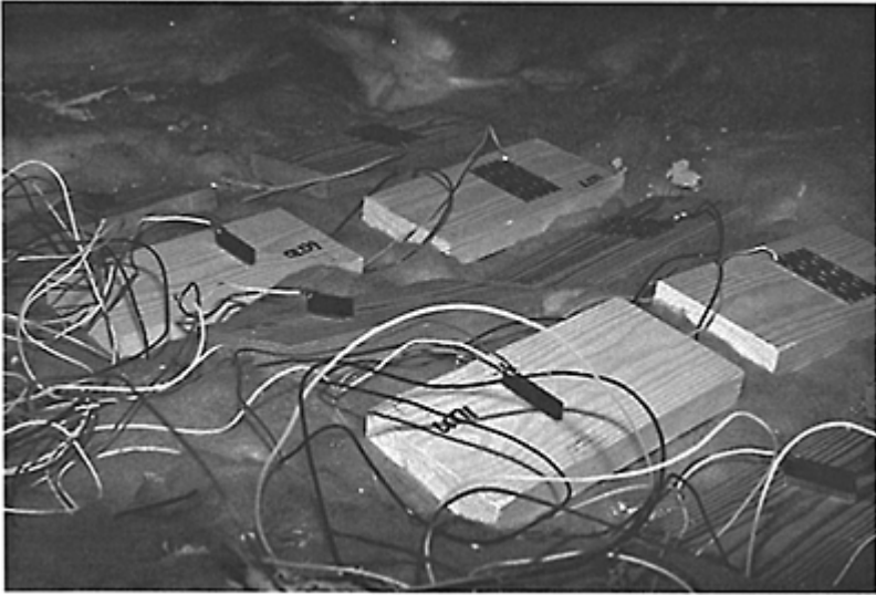
Figure 2. Timber blocks/electrodes exposed in the loft space at Liverpool.
