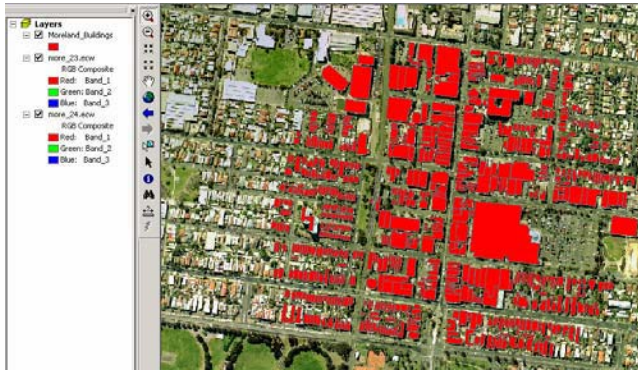
Figure 2. Building footprint data layers derived from overlaying aerial photography with cadastre boundaries, validated through fieldwork, formulated and presented in ArcMap
