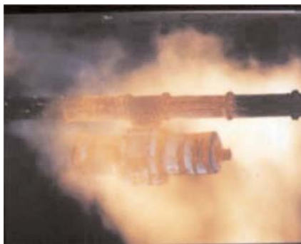
Figure 74 Jet fire example showing the high heat and pressure flame impact on a valve. Temperatures greater than 1,300°C are typical, resulting in rapid failure of steelwork.
