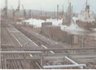
Figure 69 This example of an unignited gas release involves a ship but the same principles apply. In this case, LPG was released when a loading arm accidentally disconnected. The extent of vapour migration is clearly shown. Luckily, the cloud did not ignite.
