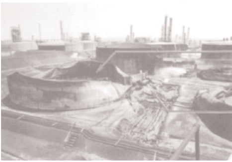
Figure 19a Tank blending of butane is thought to have caused this tank farm fire.
