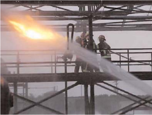
Figure 73 Bending a small jet fire on a liquid hydrocarbon loading rack (training at BP fire school).
