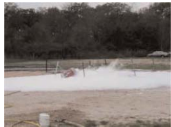
Figure 76b Another example of foam blanket over an LNG spill. This foam was applied by portable equipment, but in this case note the vapours migrating in the centre of the photograph.
