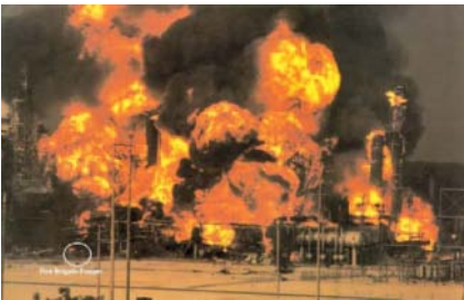
Figure 3 This fire at a refinery catalytic cracking unit started with a propane leak. The white circle on bottom left indicates the position of a fire truck where seven firefighters were killed.
