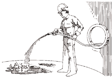
Figure 33 Pyrophoric iron sulphide must be kept wet or it will ignite.
