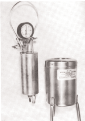
Figure 27 This is a device for determining the amount of air, or other noncondensibles, present in steam. A representative portion of the steam flows through the sample chamber, heating the sample chamber to steam temperature. Placing the sample chamber in the insulated container speeds up this step. A sample of the steam is then trapped in the chamber by closing in quick succession the inlet valve and outlet valve. The chamber is then lifted from the insulated container and cooled to 100°F (38°C). Condensation of the steam produces a vacuum in the chamber. The amount of pressure reduction is a function of the relative proportions of steam and noncondensibles (air) in the original mixture, and the air content can be calculated. This instrument cannot be used to determine concentration of air in inert gas. After purging with inert gas, absence of oxygen must be confirmed using one of several types of portable oxygen analyzers suitable for this purpose. Drawings of this analyzer can be found by contacting Amoco heritage refineries.
