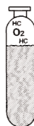
Figure 18 Propane condenses more readily into liquid under pressure, leaving the vapour space more concentrated in oxygen.
