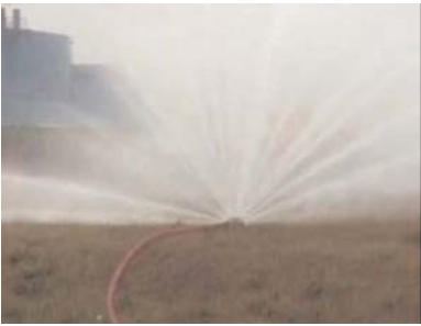
Figure 77 Example of a portable water curtain nozzle in use.
