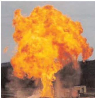
Figure 85a Typical fireballs from BLEVE events.
