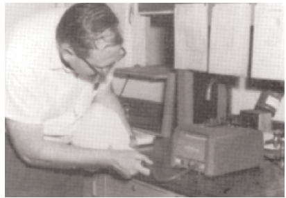
Figure 41 Vapour sample from empty LPG truck being tested for oxygen content on a portable-type oxygen analyzer.
