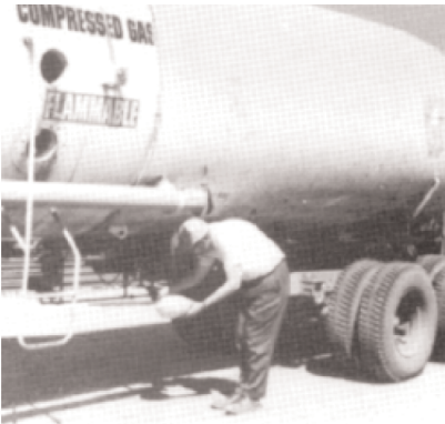
Figure 40 Vapour sample being taken from an empty LPG truck.
