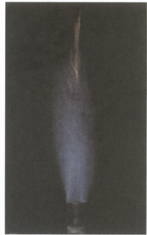
Figure 35b Good pilot flame.
