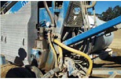
Figure 48 The operator's station, water spray pump and hydraulic lines.
