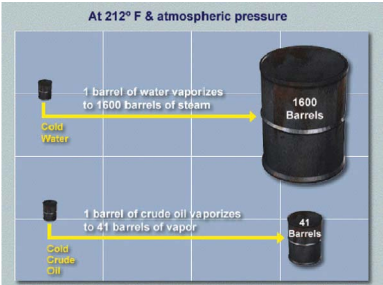
Figure 7 At atmospheric pressure, a barrel of water will flash to 1,600 barrels of steam at 212°F (100°C). A typical barrel of crude oil will flash to only 41 barrels of vapour at the same temperature.
