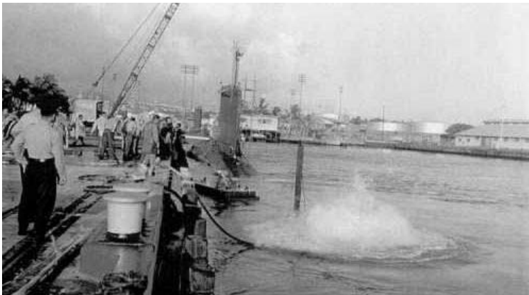
Figure 52 After portion of submarine being submerged with hatches open to kill the fire.
