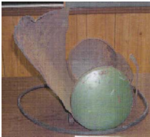
Figure 56 Air tank ruptured while being filled with compressed air.
