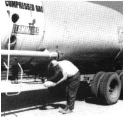
Figure 43 Vapour sample being taken from an empty LPG truck.
