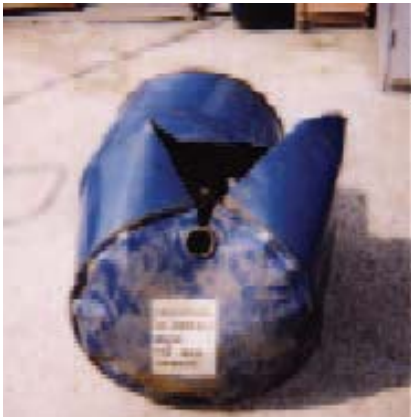
Figure 13 Damage caused to an 'empty' drum following cutting with a grinding wheel
