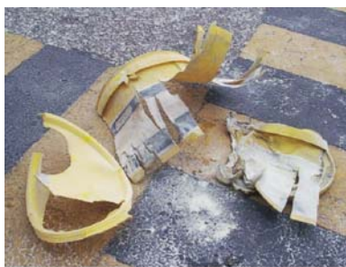
This waste collection vessel blew up, drenching the laboratory technician in kerosene.
