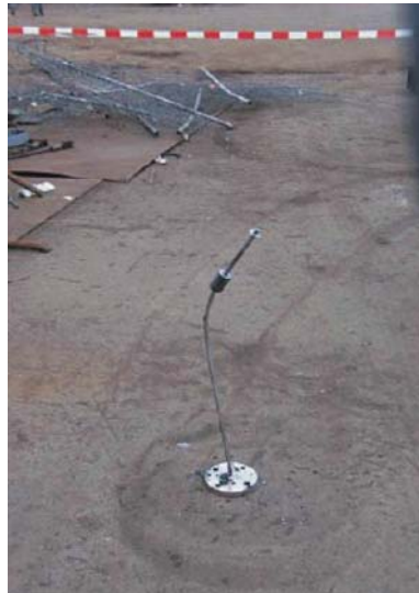
The recovered radioactive source holder
