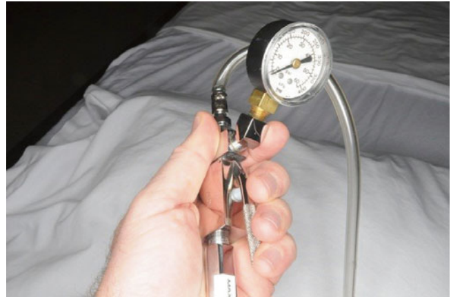
Fig. 21.8 Operate the valve 12–20 times a minute with long periods to allow gas exhalation and exchange
