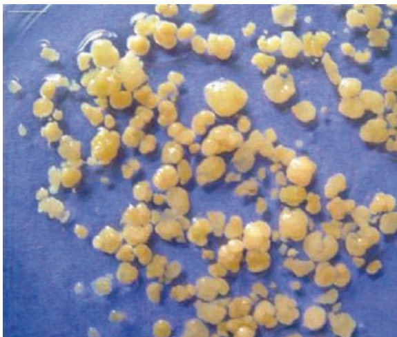
Fig. 1 Image of aerobic granules cultivated with glucose as carbon source from [48]. Scale bar = 10 mm
