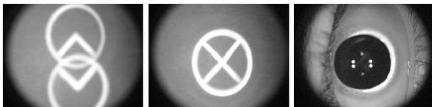
**Fig. 15.5.** Aberrometer alignment markers (*top* and *middle*) and typical scene camera image (*bottom*)
