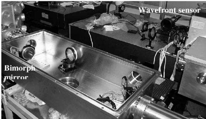
**Fig. 25.12.** Experimental set-up of AO systems at the Chinese Institute of Physics
