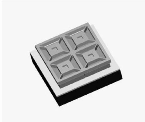
**Fig. 7.3.** Patterned actuators. The sacrificial oxide layer not shown
