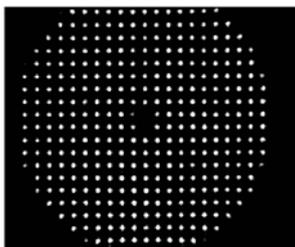
Fig. 25.5. Example of a hartmannogramme
