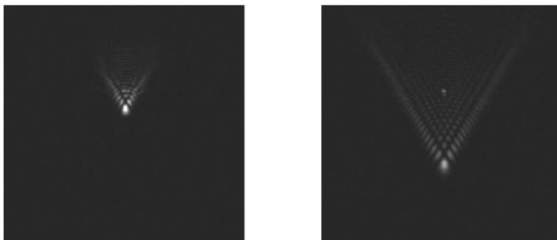
**Fig. 32.3.** Experimental aerial images for pure Zernike coma induced with the PPM. *Left:*  $C_{3,-1} = 1 \mu\text{m}$ . *Right:*  $C_{3,-1} = 3.25 \mu\text{m}$
