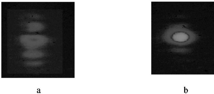
**Fig. 23.11.** Measured beam profile (a) before and (b) after optimisation using the genetic algorithm
