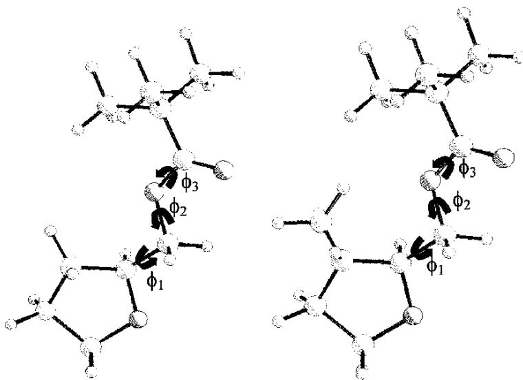
Scheme 2.10 Optimized conformational geometry of the repeating unit of PTHFM and P3MTHFM
