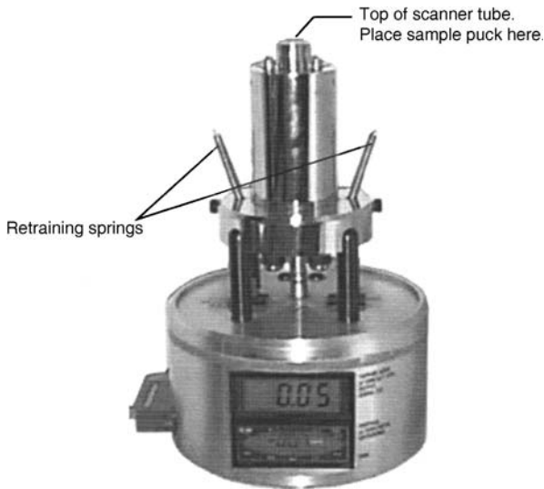
Fig. 3.15. MultiMode base with scanner mounted on support ring. Reprinted from [9, 13]
