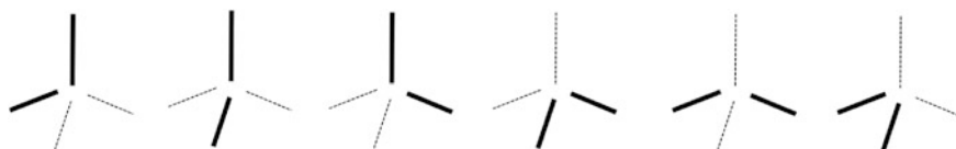
Fig. 7.26 The number of distinct ways for one water molecule to form two hydrogen bonds (solid lines) is given by 4!/(2!2!) = 6
