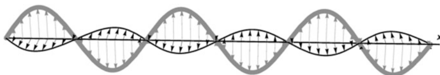
Fig. 5.27 Plane-polarized electromagnetic radiation propagating along the x -axis. The electric field oscillates in the vertical plane. Figure obtained with Mathematica
