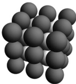
Fig. 6.28 The cesium chloride structure with the \text{Cs}^+ and \text{Cl}^- ions represented by spheres ( \text{Cs}^+ light gray spheres, \text{Cl}^- gray spheres). Figure obtained with Mathematica
