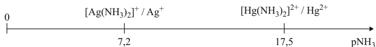
Fig. 24.3 Prediction of the ligand \text{NH}_3 exchange reaction between the couples [\text{Ag}(\text{NH}_3)_2]^+/\text{Ag}^+ and [\text{Hg}(\text{NH}_3)_2]^{2+}/\text{Hg}^{2+}
