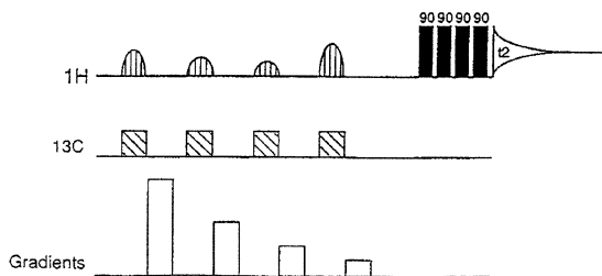
Fig. 7.28 Typical pulse sequence used for HPLC-NMR experiments
