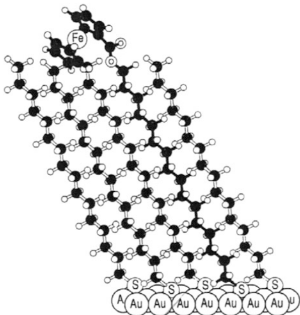
Fig. 6.17 Inferred structure of a monolayer formed by coadsorption of a ferrocene-terminated alkane thiol (highlighted with black bonds ) and the unsubstituted alkane thiol on Au(111). The conformation around the ester group is chosen to illustrate the closest approach of the ferrocene group to the electrode ( \sim 20 Å). Reproduced from [43] with permission
