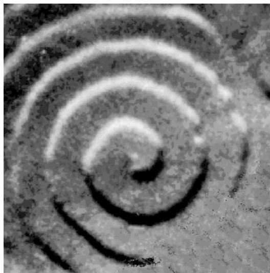
Crystallization – Spiral growth of crystals — Figure 2. Circular macro-spiral growing on the cubic face of a silver crystal, the average distance between steps being \sim 3 \times 10^{-3} cm (Courtesy of V. Bostanov, unpublished result) [xiii]
