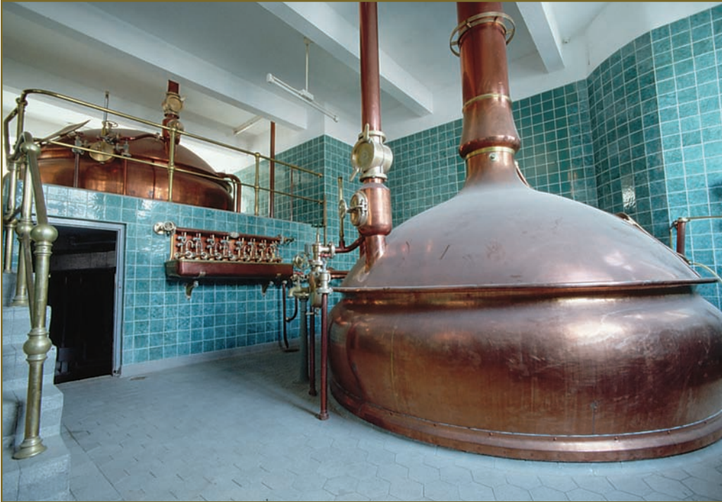
Figure 5.1 Brewing became a modern industry in 1880 when Louis Pasteur discovered the chemistry of fermentation. It then became possible to make large volumes of beverages that did not spoil during storage and shipping. The large brewing tanks shown here are specially controlled environments where yeast produces beer by fermentation.
