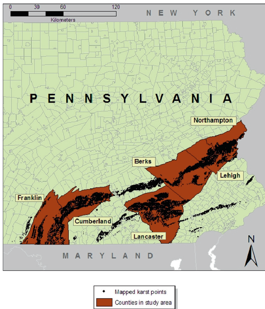
Plate 35 Mapped karst points in the six counties of the Pennsylvania study area
