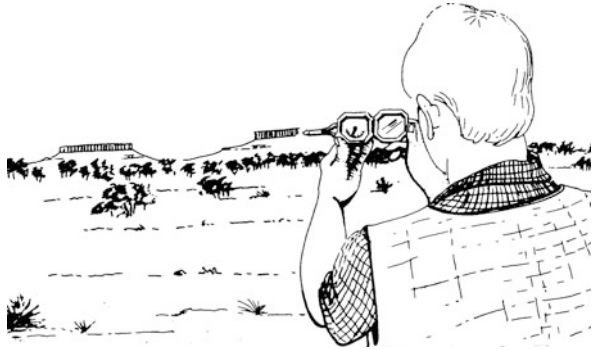
Fig. E.3 Measuring the dip of beds on a distant mesa by sighting along strike
