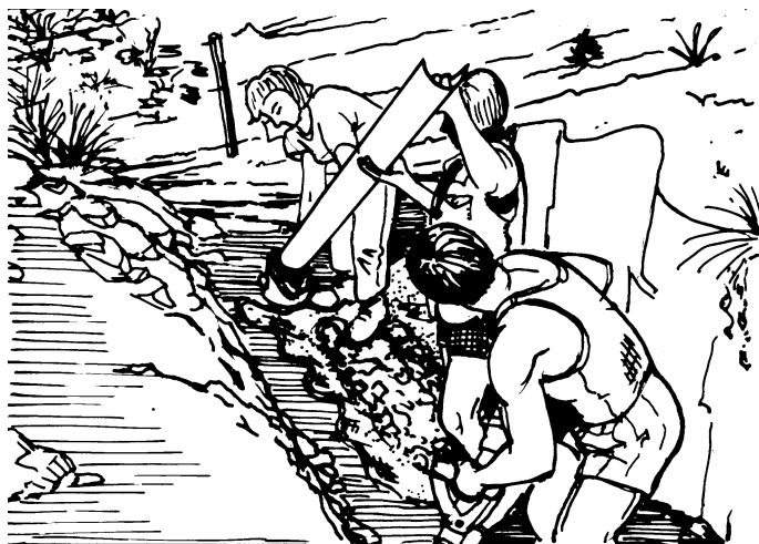
Fig. 4.5 Splitting a sample for assay from an even row of small rock fragments on the ground. The rock fragments lie on a tarpaulin; a halved length of 100 mm poly pipe is laid along the row and rocks and pipe are rolled together in the tarpaulin. Rock in the pipe is then slid into a sample bag
