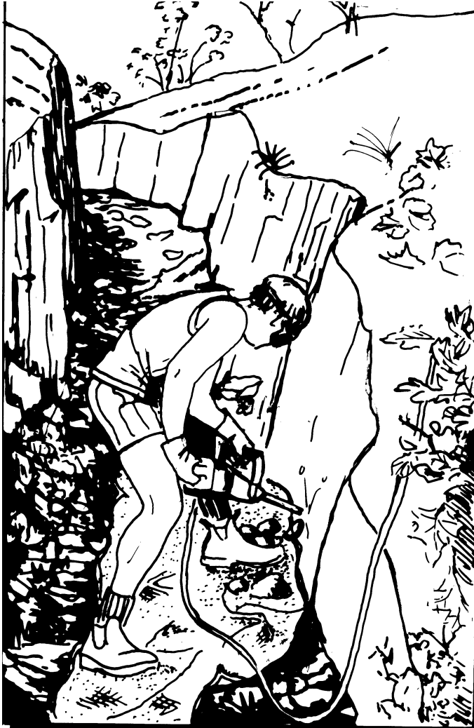
Fig. 4.4 Collecting a continuous chip-channel sample from a trench wall. The sampler is using a small electric jackhammer powered by a portable generator. The broken rock falls onto a tarpaulin laid along the trench floor. The same technique could be used for sampling any hard rock exposure in the field or in a mine
