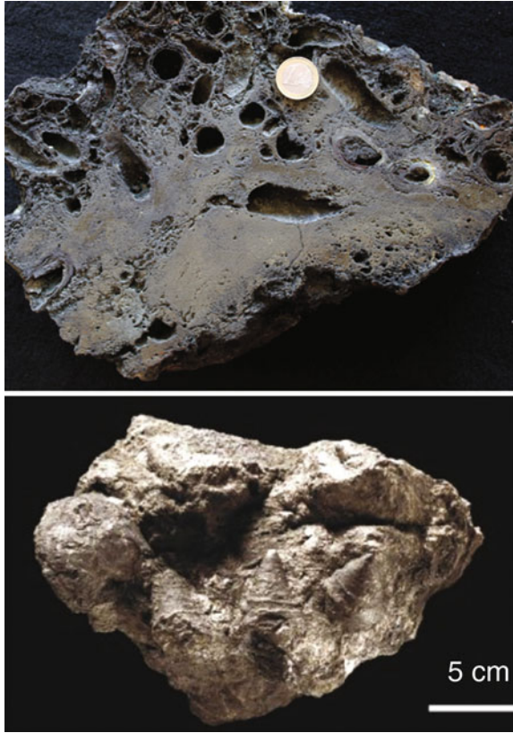
Fig. 4.9 Top photo of section cut through a chimney of a black smoker VMS-type deposit (photo N. Arndt). Bottom photo of ore from deposits in the Yaman Kasy massive sulfide deposit in the Urals. The ore contains fossilized monoplacophorans and brachiopods (photo from Phil Crabbe)
