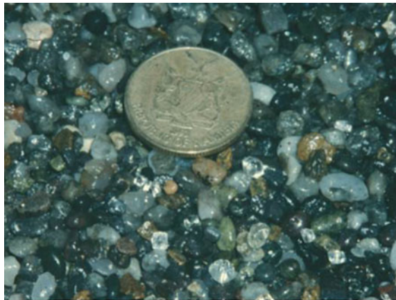
Fig. 5.4 Photos of alluvial diamonds. The top photo shows a heavy mineral concentrate of beach sediment from Namibia that contains five diamonds. Can you distinguish them from the more numerous quartz grains? Hint, the diamonds are below the coin (photo by S. Kesler). The bottom photo shows a group of gem quality diamonds that have been picked out of a beach gravel (photo from www.diamondfields.com )
