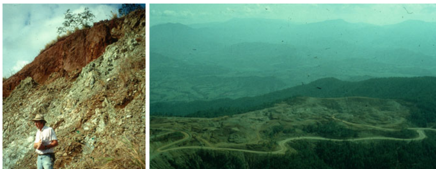
Fig. 5.11 Left Thin layer of iron-rich nickel laterite overlying serpentinite at the Guanajibo deposit, Puerto Rico. Right Air view of nickel laterite mine, Bonao, Dominican Republic showing extensive surface disruption caused by mining shallow deposits such as laterites (photos by S. Kesler and M. Seaward)
