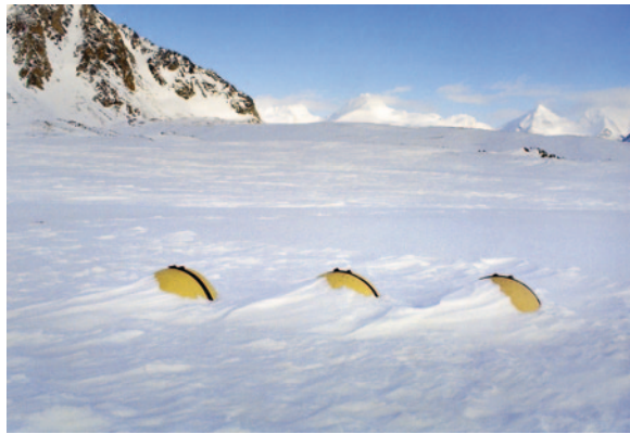
Fig. 2.4 Site 13 (BJ) of the HSP station with three dome-shaped boxes containing seismographs
