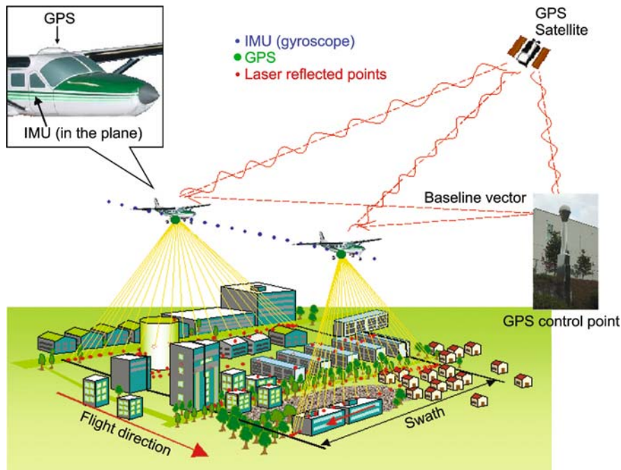
Fig. 17.3. Concept of the airborne LIDAR
