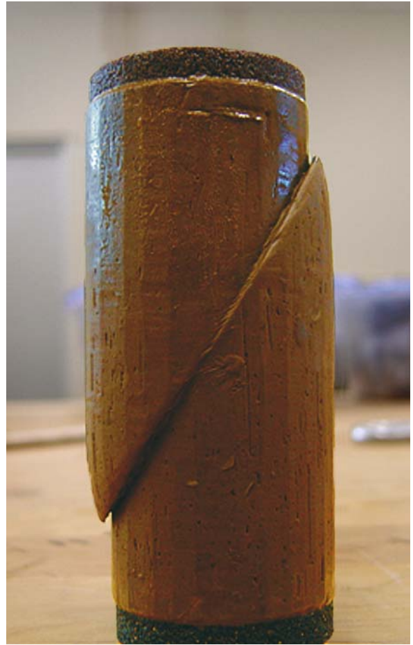
Fig. 9.10. Pre-cut soil specimen after shearing in triaxial compression
