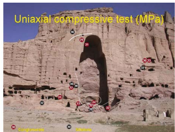
Fig. 25.12. Uniaxial compressive tests from point load in both conglomerate and siltstone
