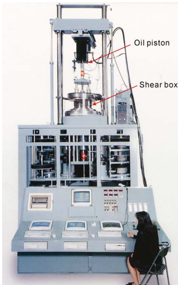
Fig. 6.2. Photo of the undrained dynamic-loading ring shear apparatus (DPRI-6)
