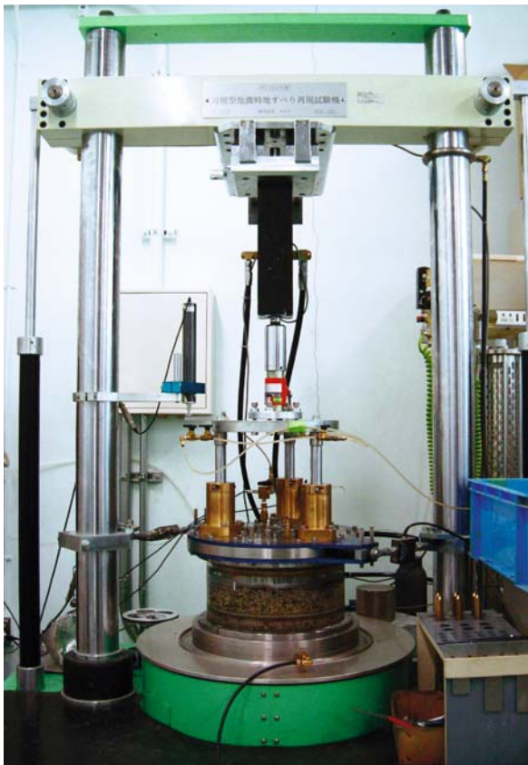
Fig. 7.1. Overview of the ring shear apparatus with a transparent shear box (DPRI Ver.7)
