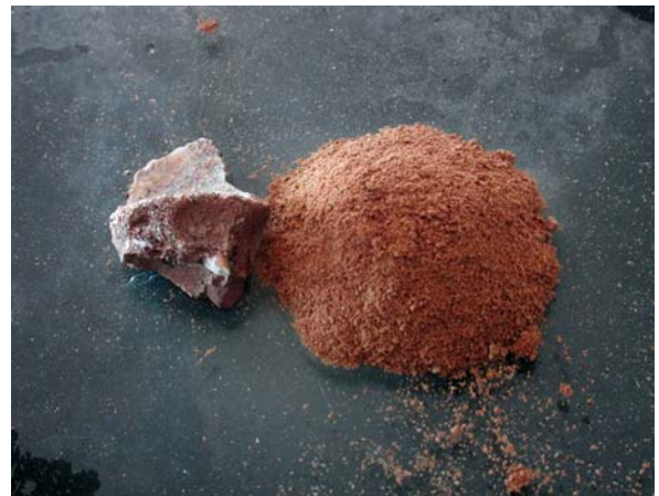
Fig. 25.6. Stability of conglomerate (right) and degradation of siltstone (left) when weathered, after only few minutes of submersion in water
