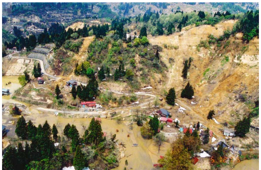
Fig. 21.17. Successive slope failure caused by snowmelt. At the main scarp (Higashi-Takezawa)
