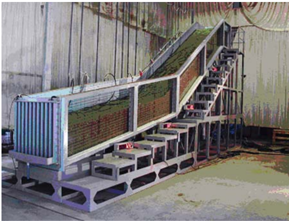
Fig. 15.2. The flume before collapse
