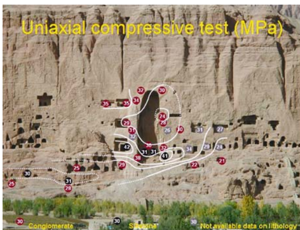
Fig. 25.11. Uniaxial compressive strength from Schmidt hammer field survey
