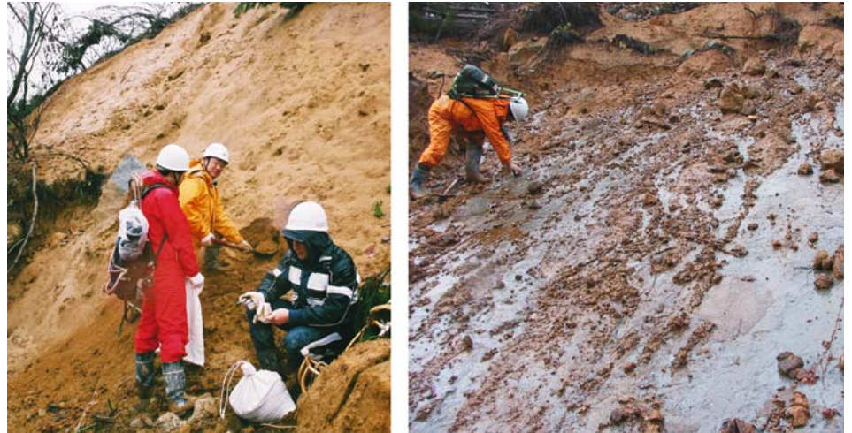
Fig. 14.11. Sampling from the sand layer (left) behind the sliding surface and over the stiff silt layer (right)
