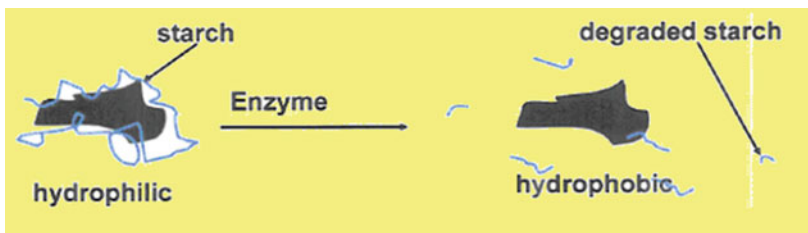
Fig. 9.2 Schematic diagram showing mechanism of Amylase action on fiber. Mohammed (2010); Reproduced with permission
