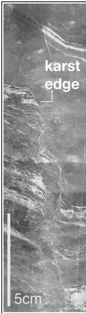
Figure 11.15. Typical multistage dissolution collapse and fill in Maha Sarakham Fm. by chevron halite. Cavities are sometimes filled by clear sylvite, not halite.
