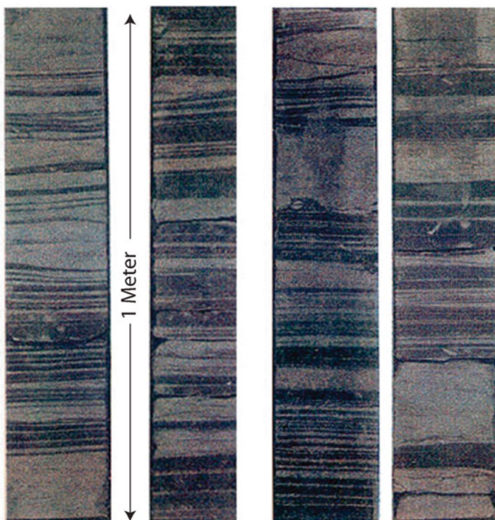
Fig. 6.14 Laminated sandstones interbedded with shales in this core are difficult for conventional logs to evaluate, as resolution of the resistivity tools are not high enough. This interval may well appear to be a shale or siltstone on a GR or resistivity log. Photo courtesy of Bernd Herold
