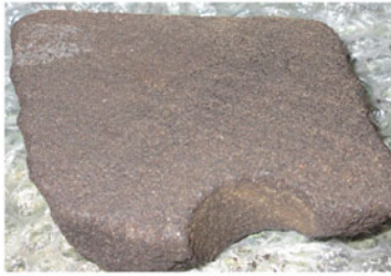
A. Heavily stained 'super perm' coarse-grained Tertiary fluvial sandstone, India. Porosity > 20%, permeability > 1000 md
