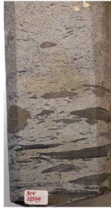
B. Spotty stain in low permeability Jurassic tidal channel sandstone, Russia. Porosity 10-15%, permeability 5-30 md
