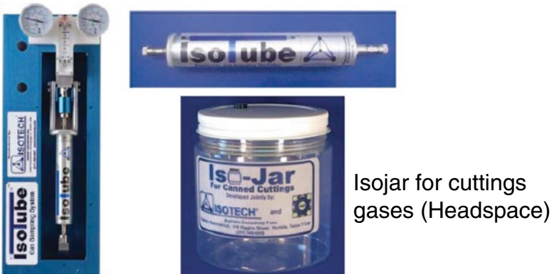
Fig. 8.27 Mud gas sampling methods. From Ferworn et al. (2008). Reprinted with permission
