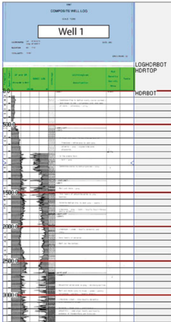
Fig. 3.10 Example of a scanned image of a well log that has been depth registered in a workstation (left). On the right are hand-digitized lithologies captured from the logs and text on the original raster. These interpreted lithologies are stored as ASCII curve data, and subsequently be used for calculations or display in cross-sections
