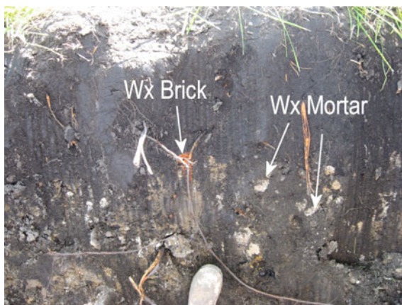
Fig. 5.2 Weathered brick and mortar in 100 year-old demolition site anthrosoil
