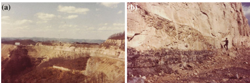
Fig. 9.3 Strip mining as it was carried out in southwestern Virginia during 1976: a "Shoot-and-shove" method produced multiple benches and large-scale devastation of the landscape. b Overburden and coal have been removed leaving a narrow bench and "high wall" ~15–20 m in height. Photos by J. Howard
