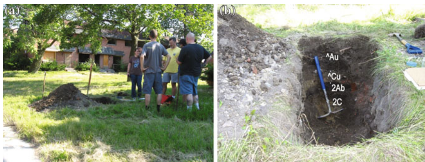
Fig. 1.2 Profile of neogenetic anthrosoil at former demolition site: a previous site was demolished before construction of building (derelict) in 1942; b anthropogenic soil profile developed in fill overlies buried natural soil. Photos by J. Howard
