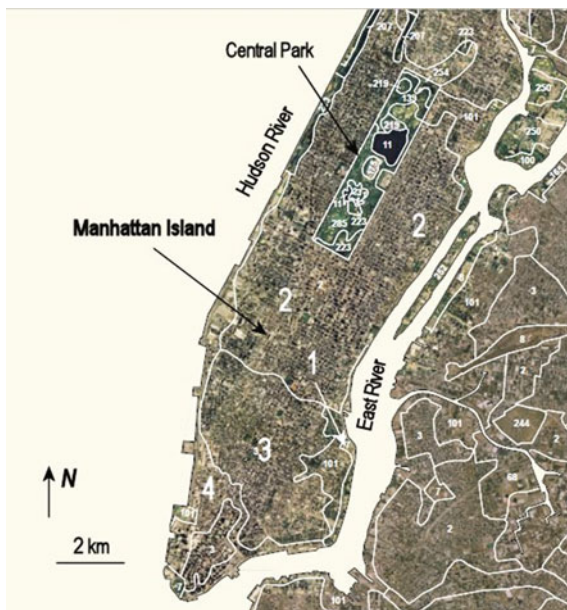
Fig. 10.2 Reconnaissance soil survey of New York City (Soil Survey Staff 2005). Map units 1–4 comprising most of Manhattan Island are manufactured land
