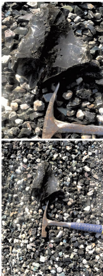
Fig. 10.12 Steel-making slag near Baden, Pennsylvania, USA. Fragments range from metalliferous, with basalt-like appearance, to a glassy and obsidian-like. Photos by Russell Losco
