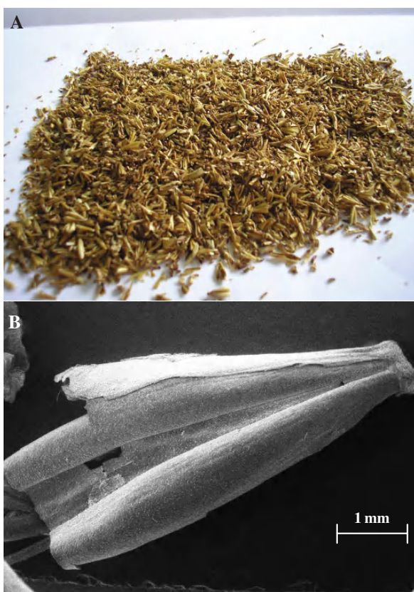
Fig. 16.2 Appearance of spent grains (A) and micrograph by scanning electron microscopy (B) with 45-fold magnification (Mussatto et al. 2006b)
