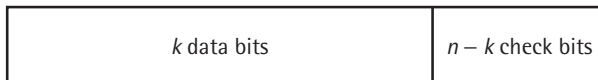
Figure 7.15 An n -bit codeword with k data bits and n - k check bits.
