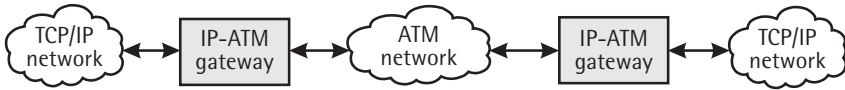
Figure 8.1 Two TCP/IP subnets are connected through an ATM network using IP-ATM gateways.
