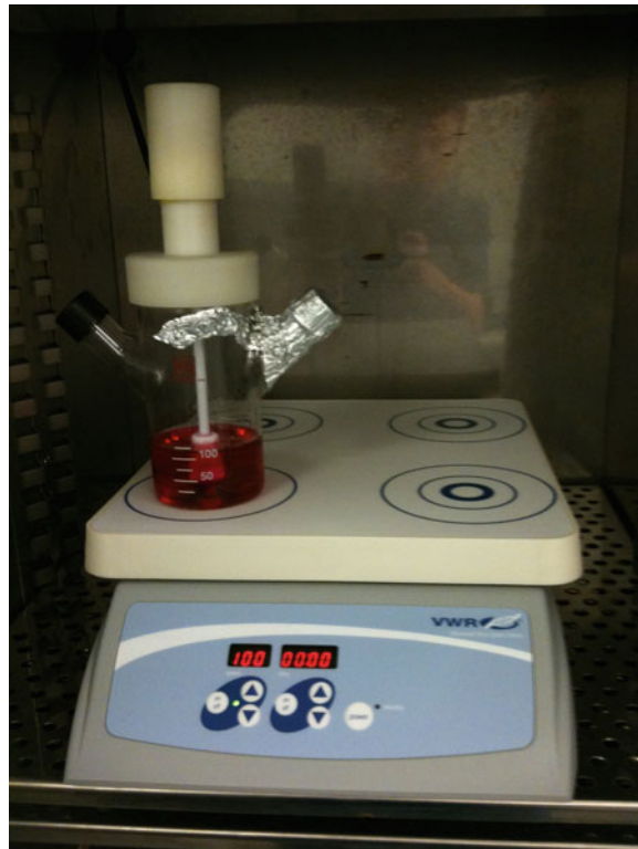
Fig. 1. Stirred suspension bioreactor setup in 37°C CO 2 incubator. The 100 ml bioreactor is placed on the magnetic stir plate and the speed is set and confirmed (see Note 8) at 100 rpm.
