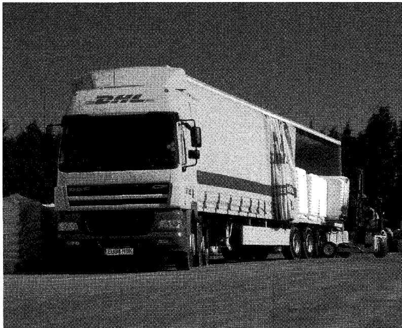
Figure 23.10 Curtain-sided trailer giving ease of access to the load (courtesy of Daf Trucks)
