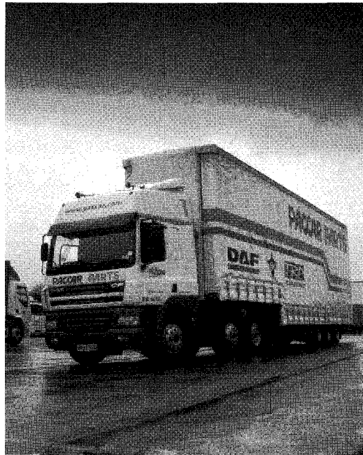
Figure 23.4 An articulated vehicle featuring a double-deck trailer (courtesy of Daf Trucks)
