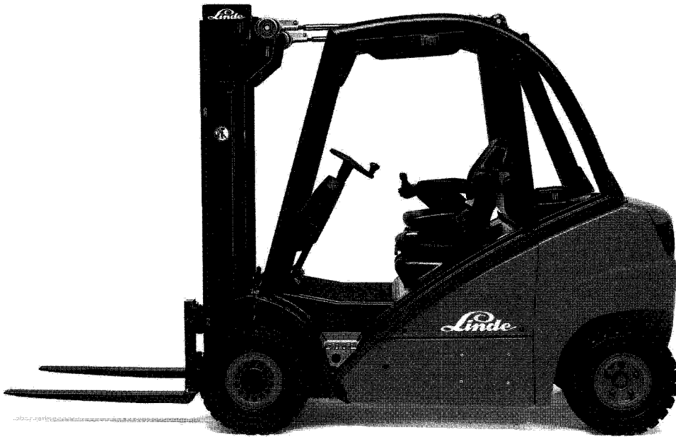
Figure 15.3 Counterbalanced fork-lift truck (courtesy of Linde)
