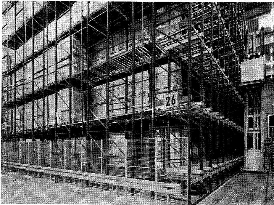
Figure 15.10 Pallet live storage (courtesy of Jungheinrich)
