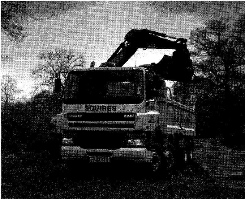
Figure 23.5 An eight-wheeled rigid tipper vehicle (courtesy of Daf Trucks)
