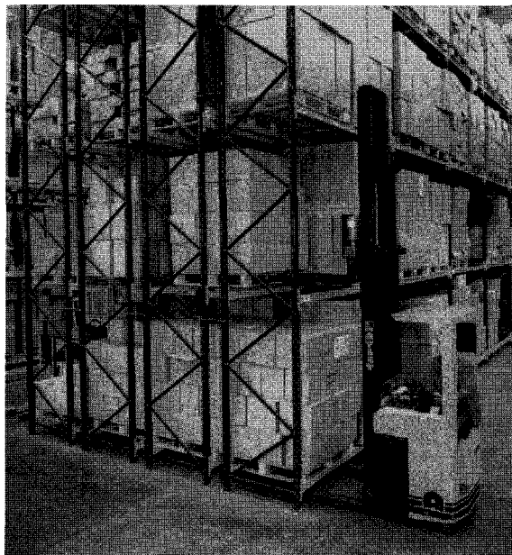
Figure 15.7 Double-deep racking (courtesy of Link 51)
