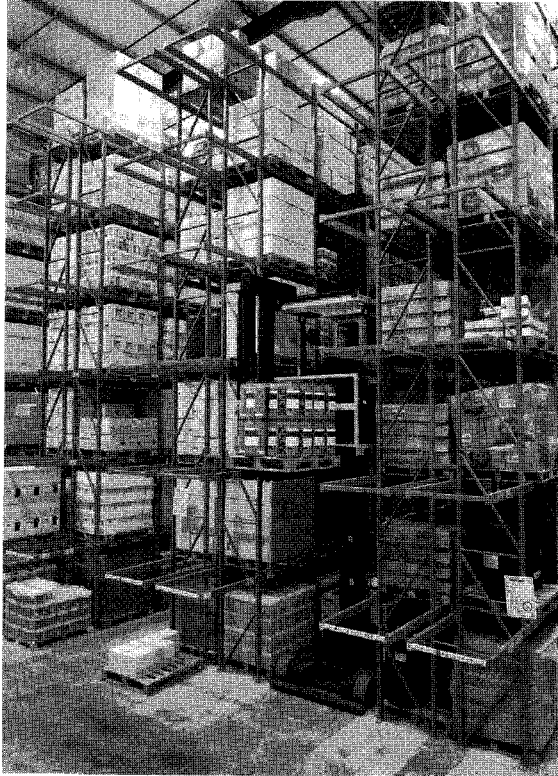
Figure 15.8 Narrow-aisle racking (courtesy of Redirack)
