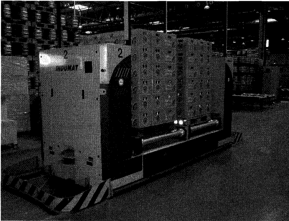
Figure 15.1 Automated guided vehicle (courtesy of Indumat)
