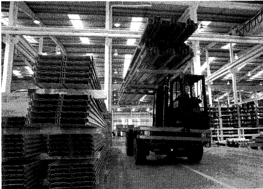
Figure 16.5 Side-loader (courtesy of Linde)
