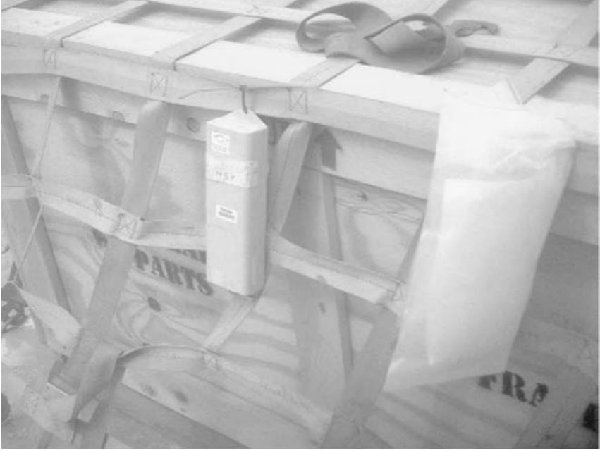
Figure 4.5 Radio frequency tag attached to an Air Force 463-L pallet.
